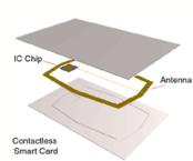
Internal components of a Mifare contactless smart card.
