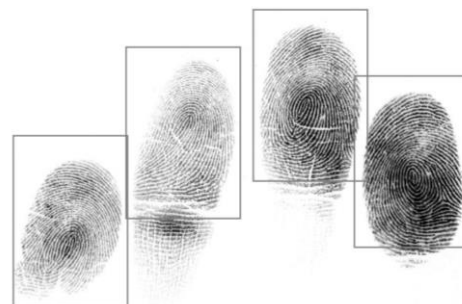
The Bioidentidad FS64 performs the automatic detection of each individual finger in simultaneous
