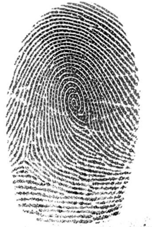
The fingerprint obtained with the FS83C is of such high quality that even the pores located on the finger ridges can be seen.
