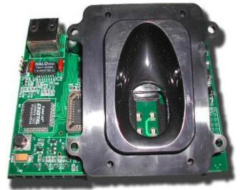
The FS83C biometric fingerprint module is internationally recognized for its high quality, which has been certified by the FBI. It is designed to be conveniently integrated with any hardware via ethernet or serial interface.
